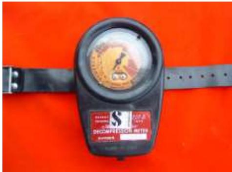
The SOS Decompression Meter (D.C.P.) was introduced in 1959 by the Italian firm, SOS Diving Equipment, Limited and became the first commercially successful decompression meter. It used a ceramic filter between two chambers to estimate nitrogen absorption and off-gassing in the diver. The meter was initially marketed in the United States by Healthways and then by Scubapro beginning in 1963 and continuing until the late 1970s.
